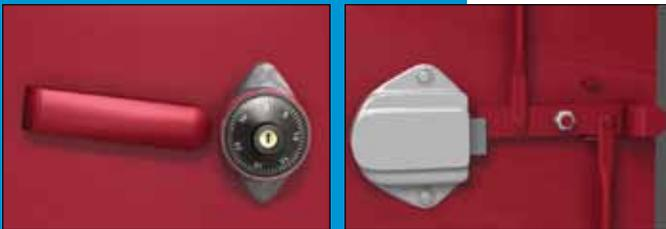
The cremone latching system provides extra security by using the principles of a fulcrum to transfer the rotary motion of a handle-turn into the vertical actuation of two positive-action locking bolts that engage with the frame at the top and bottom of the door, and a center latch engaging at the side.
