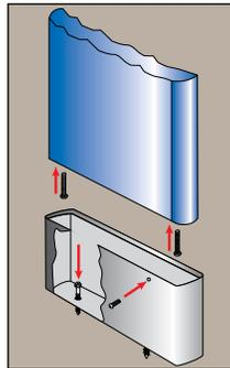
**Easy-Stall Shoe** for floor anchored/overhead braced. Stainless steel, type 304 mounting shoe. Easily adjusted leveling bolt. True concrete anchor screws designed for lasting holding power. Anchor rated at 2770 lbs. pullout strength.
