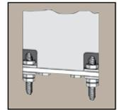
**Floor Stud Mounting System** for floor and ceiling anchored. Attach mounting system, insert pilaster and adjust height and level by turning the lock nut adjusters.
