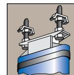
**Alternate Pilaster Mounting**
