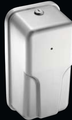
20365 AUTOMATIC FOAM SOAP DISPENSER A foam drop is dispensed out of the nozzle on unit bottom each time its battery-operated sensor is activated. Capacity: 34 oz. (1000 ml) of liquid foaming soaps within a wide range of viscosity. Overall size: 5½" x 10⅞" x 4" (140 x 276 x 102 mm) projection.
