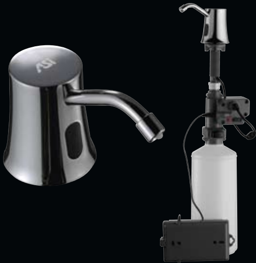
20333 AUTOMATIC DECK MOUNTED SOAP DISPENSER Constructed of polished type 304 stainless steel on exposed surfaces with battery-operated, hands-free sensor. LEDs indicate function, battery condition and soap supply level on face front. Translucent tank. Capacity: 54 oz. (1600 ml) of liquid soap.
