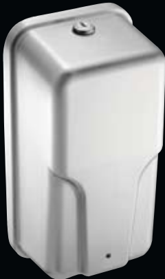
20364 AUTOMATIC SOAP OR HAND SANITIZER DISPENSER Hands-free, battery-operated soap or hand sanitizer dispenser. Dispensing cycles adjustable with tamper proof magnetic key. Seamless drawn type 304 stainless steel cover. Translucent removable internal tank for easy-to-view level. LED indicates adjustment and operation. Capacity: 34 oz. (1000 ml). Overall size: 5½" x 10⅞" x 4" (140 x 276 x 102 mm) projection.
