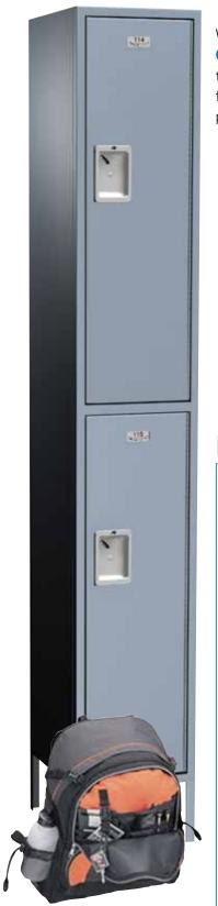
With the same standard features as the Traditional line, the Traditional Plus **Collection** is intended for more rugged applications. Available in single-, double- or triple-tier configurations, this collection features 14 gauge doors with 16 gauge full-height reinforcement channels, frame-secured 11 gauge frame hooks with protruding padlock hasps, and a maintenance-free, single-point latching system.
